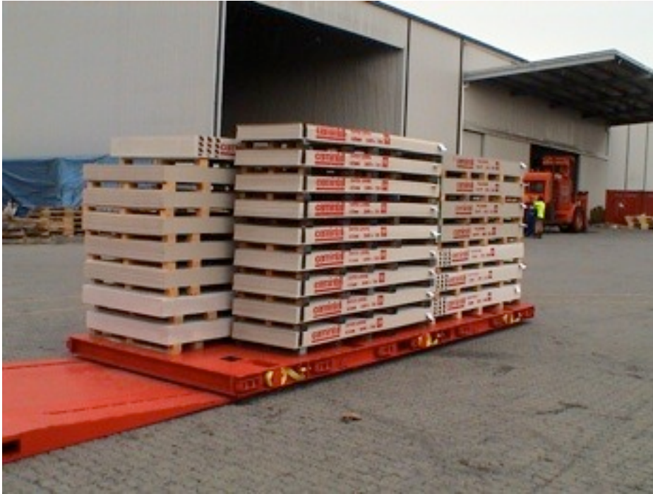
The SLC is loaded off the ramp and then pushed up the ramp and into the container.
